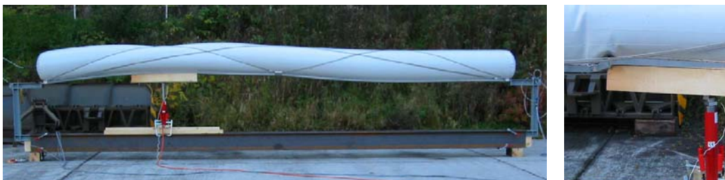
Figure 7. Limiting load test of the Tensairity beam with 8 m span. Deformation of the beam at the maximal applied load of 35 kN shortly before failure (left). Shear failure of the compression element (right).
